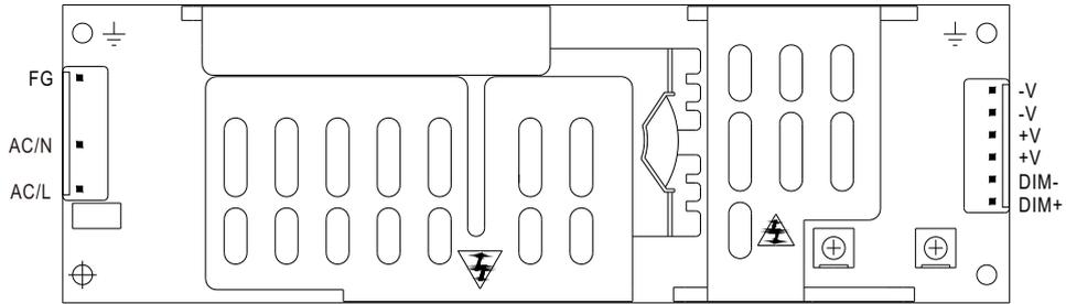
※ Built-in 3 in 1 dimming function, output constant current level can be adjusted through output connector by 1~10VDC, PWM signal, or connecting a resistance between DIM+ and DIM-.
