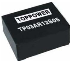
**DESCRIPTION: 3W 2.5KV Isolation Wide Input AC/DC Converters**
