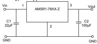
C1: A low ESR capacitor is required to keep the converter to a minimum.
