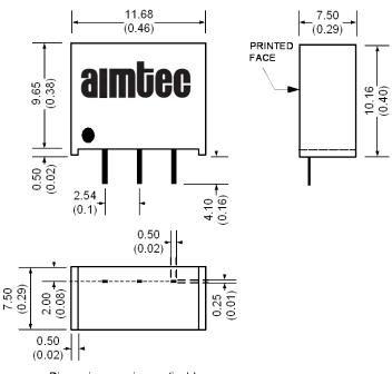
Dimensions are in mm (inch) Pin Pitch Tolerance: 0.35 mm (0.014 inch) Case Tolerance: 0.50 mm (0.02 inch)
