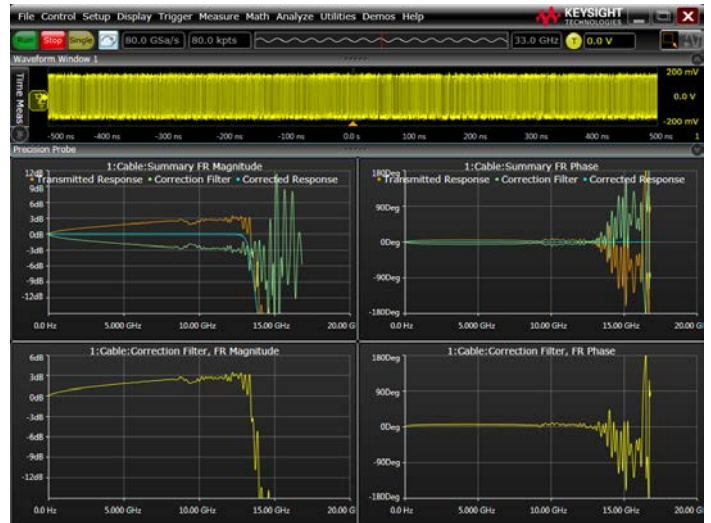
The magnitude and phase response of a cable corrected using PrecisionProbe.
