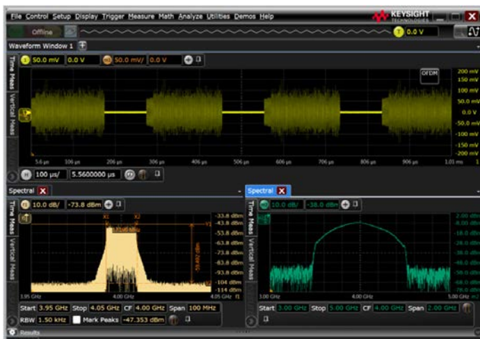
Use Infiniium capture and analysis of radar bursts as shown in this orthogonal frequency-division multiplexing (OFDM) example.
