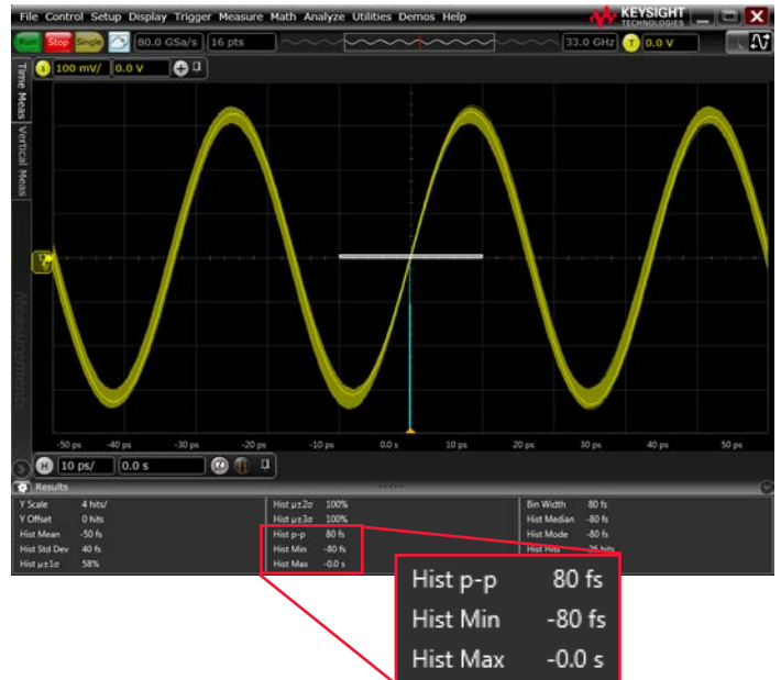
Jitter measurement floor of less than 100 fs (80 fs with 30 GHz input sine wave).
