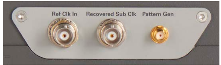
External reference clock input is one of the methods to enable SSC tracking by the hardware serial trigger.
