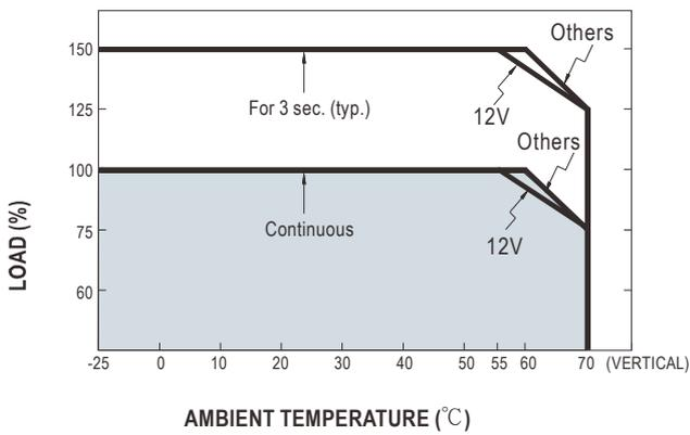
■ Output derating VS input voltage
