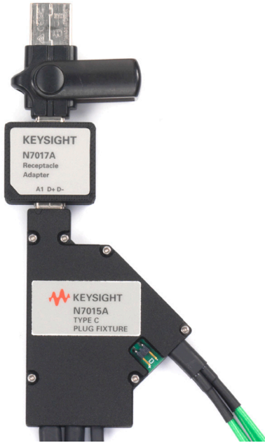
Figure 11. With the use of the N7017A receptacle adapter, the N7015A test fixture can act as a receptacle fixture.
