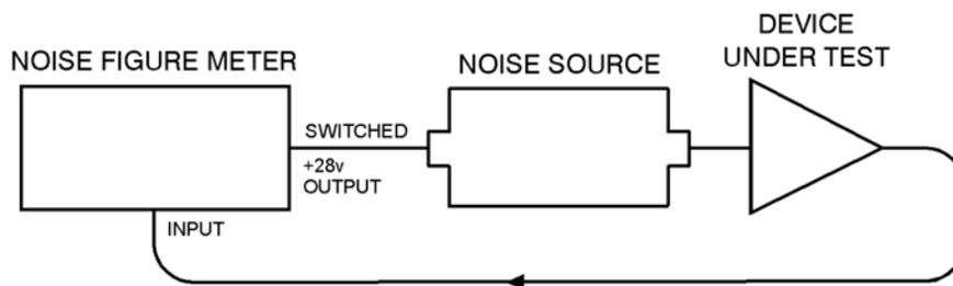
**Figure 4-1** Typical noise figure measurement test setup
