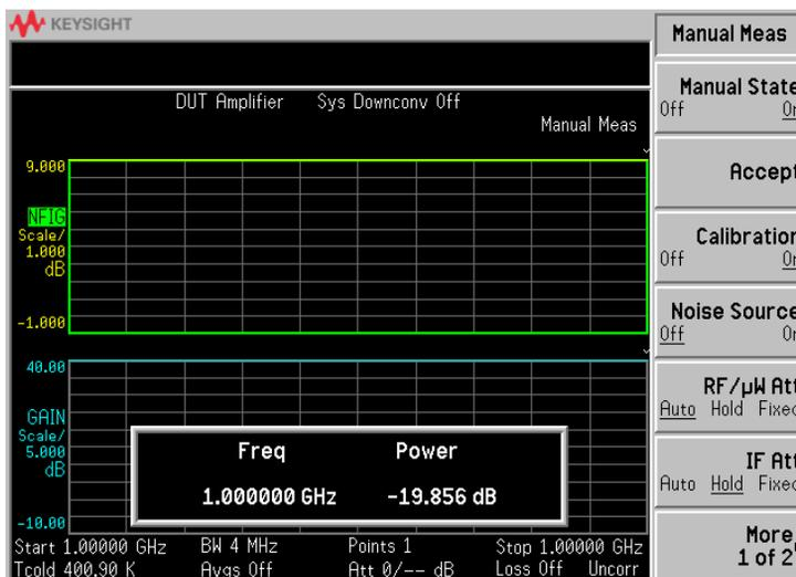
**Figure 4-6** Typical example of power reading with Noise Source Off
