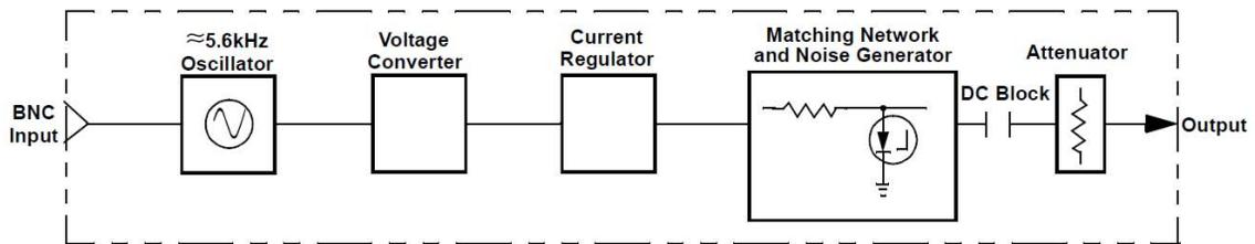
**Figure 4-8** Simplified diagram of the noise source
