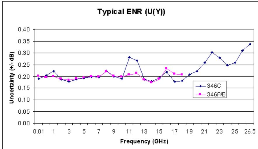
**Figure 3-1** Characteristic<sup>[1]</sup> ENR plot versus cardinal frequency points
