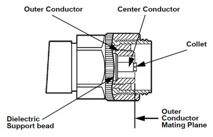
Figure A-1 Precision 7 mm connector
