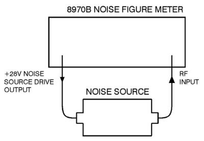
Figure 4-3 Operator's check test setup 2a
