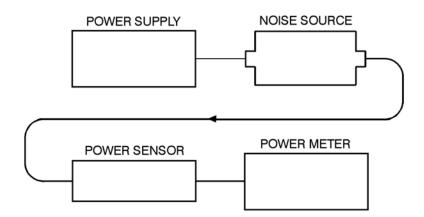
Figure 4-2 Operator's check test setup 1
