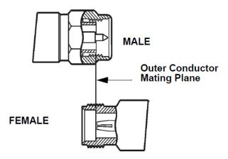
Figure A-2 Precision 3.5 mm connectors
