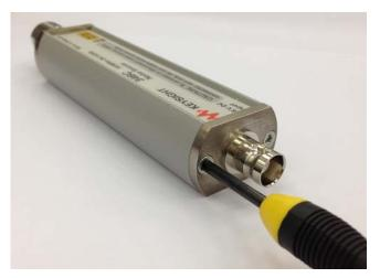
Figure 4-7 Preparing for parts removal/replacement
