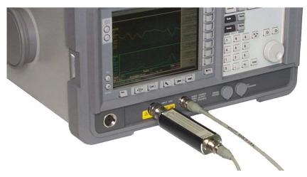
Figure 4-4 Operator's check test setup 2b
