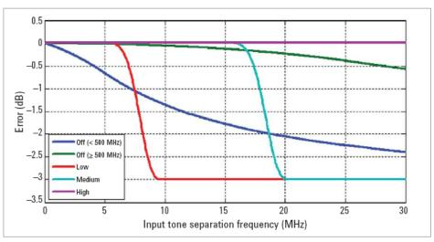
Figure 2. U2021XA/22XA error in peak-to-average measurements for a two-tone input (High, Medium, Low and Off Filters)
