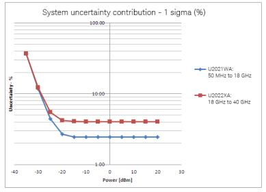
Note: The above graph is valid for conditions of free-run operation, with a signal within the video bandwidth setting on the system. Humidity < 70 %.
