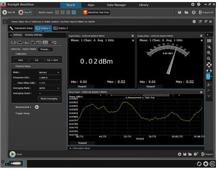
Figure 3. Digital meter, analog meter and datalog view
