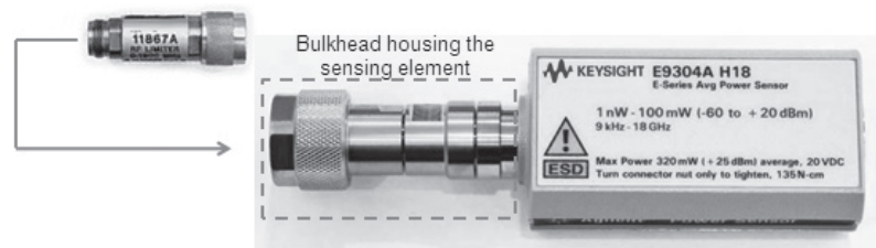
Figure 2. The bulkhead of a power sensor
