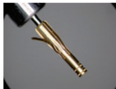
Figure 10. Damaged female connector fingers
