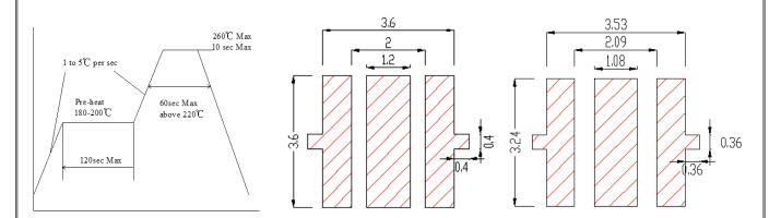
**Recommended Reflow Soldering Condition** (Lead-free solder)
