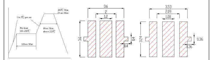
**Recommended Reflow Soldering Condition** (Lead-free solder)
