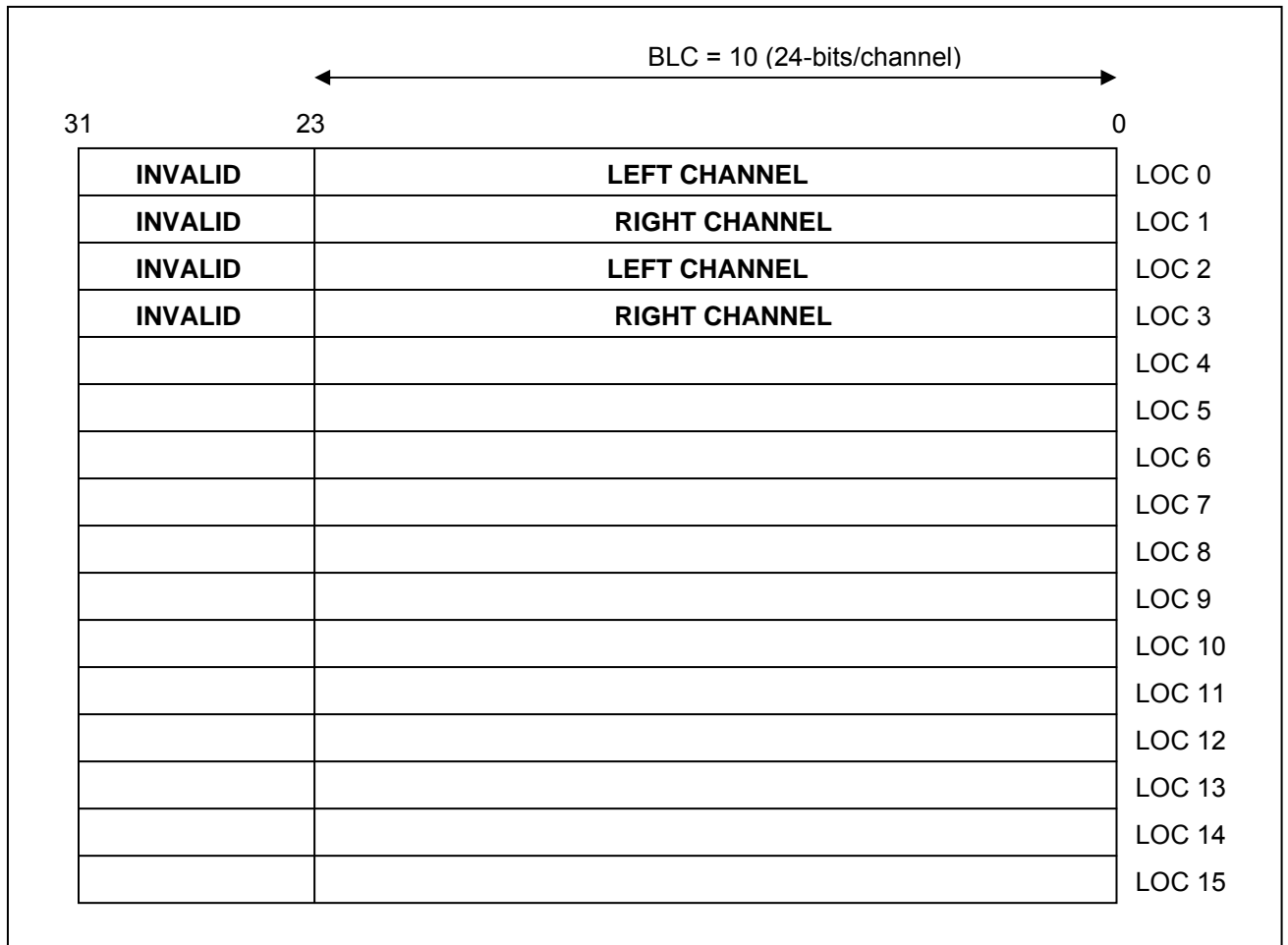
Figure 36-5. TX FIFO Structure for BLC = 10 (24-bits/channel)
