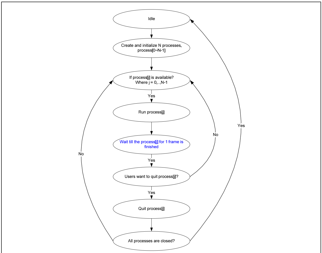
Figure 21-5. Codec firmware state diagram
