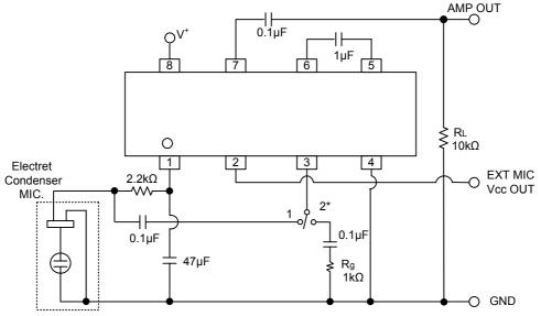
\*SW 2 :Output Noise Voltage Test
