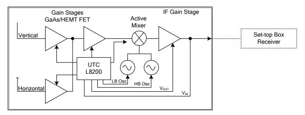
Polarization and band switching on the UTC **L8200** uses the standard 13~17V and 22kHz as defined by Astra. The exception is that the devices voltage detector has a much tighter tolerance than required to increase field reliability.
