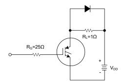
Fig 1. INDUCTIVE SWITCHING TEST CIRCUIT
