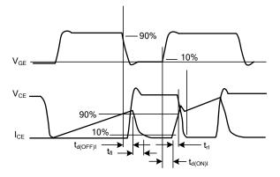
Fig 2. SWITCHING TEST WAVEFORMS
