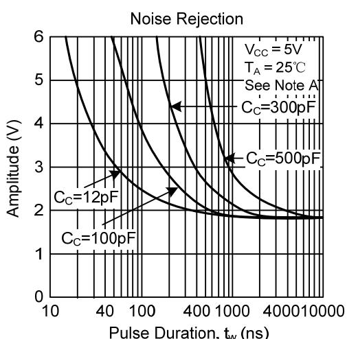
The maximum amplitude starting from 0V of a positive-going pulse that will not cause a change in the output level.
