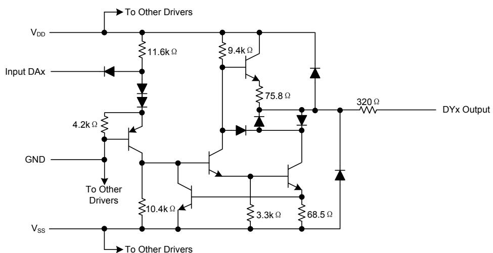
CIRCUIT OF EACH RECEIVER (Resistor value shown are nominal.)
