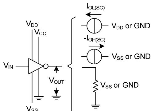
Figure. 1 For  $V_{OH}$ ,  $V_{OL}$ ,  $I_{OH(SC)}$ ,  $I_{OL(SC)}$
