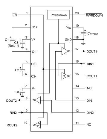
Notes: 1. C3 can be connected to  $V_{\text{CC}}$  or GND.
