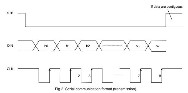
Because the DIN/DOUT pin in a bi-directional pin, it is recommended to connect an external pull-up resistor to this pin (1 K $\Omega$  to 10 K $\Omega$ ).
