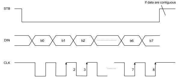
Fig 1.Serial communication format (reception)
